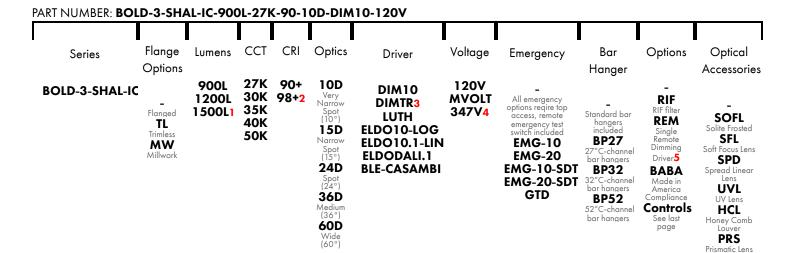
Any fixture can take maximum 2 Optical Accessories 1 The highes lumen will not be compatible with any optical accessories 2 98 + CRI is available only on 27K, 30K and 40K 3 DIMTR is only available with 120V 4 347V is only available with DIM10 5 Remote mount Maximum distance from light fixture to remote power supply is 100' using 14 gauge wire, 50' using 16 gauge wire
